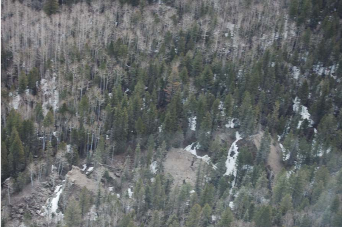
Figure 9. Aerial view of the rockfall channel just above the recent landslide. The main surface drainage for the landslide goes through this area and is still somewhat snow covered. Large vertical cliffs are uphill from this point by ¼ mile. This area is a large collection point for water and is very well shaded by the cliffs.
