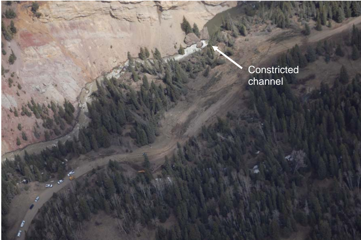
Figure 3. Aerial view of the landslide toe affecting the East Fork of the San Juan River. Note the cliff-face across the river exposing Tertiary Volcanic bedrock.
